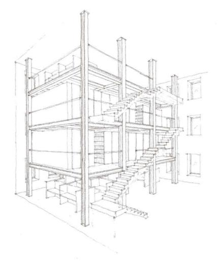
infill beams, W24x68 or W24x76 girders to transfer the library columns above, and 2  $\frac{1}{2}$ -inch stone weight concrete over 3-inch composite metal deck. Also, the existing walls needed additional lateral support after losing the fourth and fifth floors. The engineers reinforced them with 14x6 HSS tubes tied back to the existing floors.
